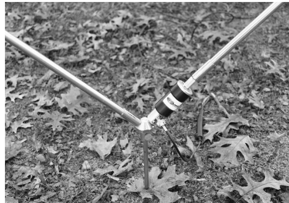
Plate 3. Installed Inverted Delta Loop Configuration.
