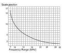
This chart is indicative and refers to a standard adjustment scale that may change depending on each site and installation method. offers indicative lt only measurements.
